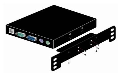
Figure D-1: Rack Mount Installation Diagram
